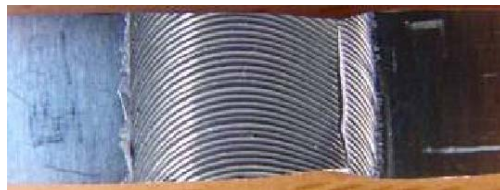
Fig. 2 Crack path of AA6082-T6 FS welded specimen.
