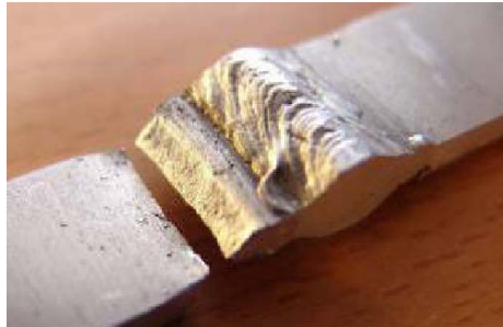
Fig. 1 Fracture surface of a MIG welded specimen of AA6061-T6.
