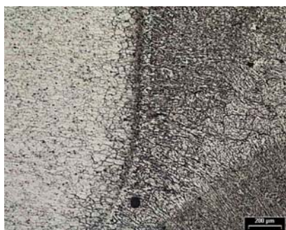
(c) Microstructure 3, limit of the weld bead
