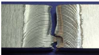
(a) AA6082-T6 FS welded fatigue tested specimen, fracture location
