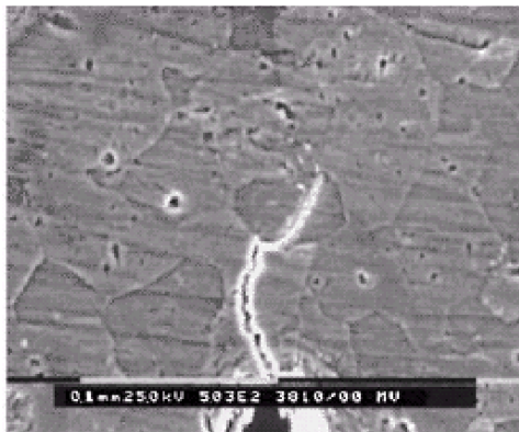
Fig. 1 Arrested fatigue crack by grain boundary in 2024-T351 aluminium alloy.
